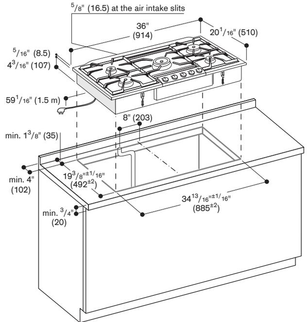
Minimum distance from the appliance cut-out to the side wall  $11\frac{13}{16}"$  (300 mm).
