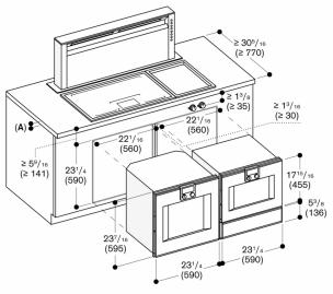
A: Min. worktop thickness  $^3/_4$  " (20 mm) for surface-mounted installation,  $1^3/_{18}$  " (30 mm) for flush installation
