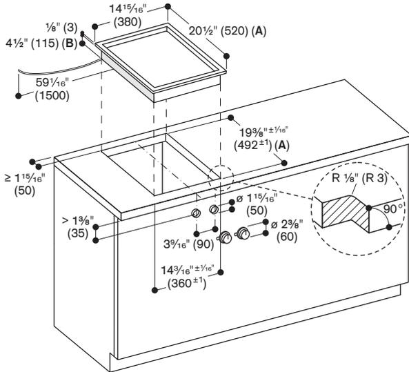
Minimum countertop thickness  $\frac{3}{8}$ " (20 mm) for surface mounted installation. See separate planning notes on page 104.
