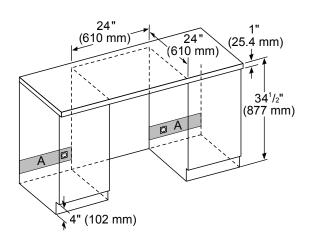
Recommended area for installation connection - a 2<sup>1</sup>/2" (63 mm) diameter hole is recommended. Location of power cord at base of the appliance.
