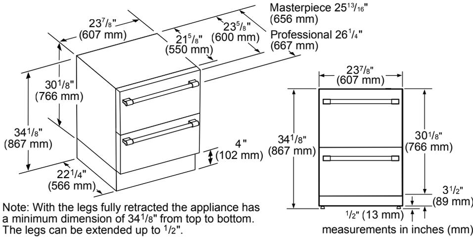
Note: With the legs fully retracted the appliance has a minimum dimension of 34<sup>1</sup>/<sub>8</sub>" from top to bottom. The legs can be extended up to 1/2".
