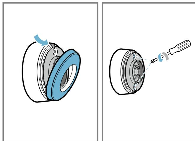
2. Open the cooking sensor cap and remove the battery from the base.
