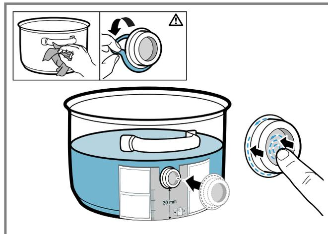
3. Press down all over the surface of the silicone patch, including in the center.
