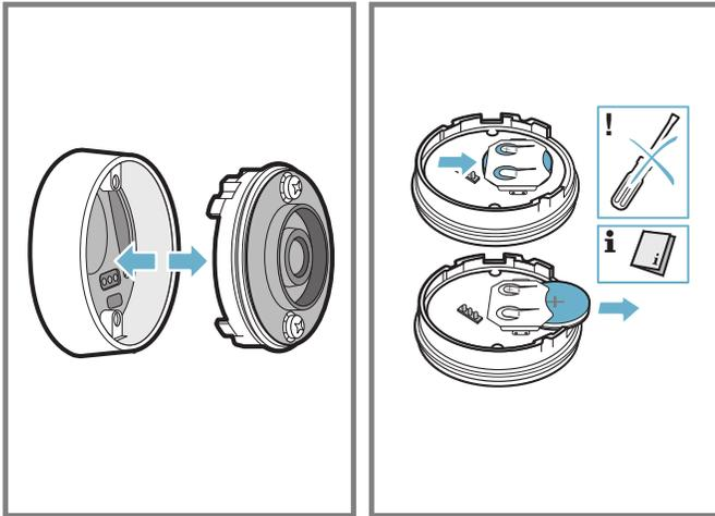
3. Insert a new battery, observing the instructions for the battery poles. Only use premium-quality CR2032 batteries.
