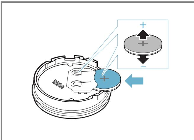
**Note:** Do not use any metal objects to remove the battery. Do not touch the battery terminals.
