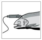
Turning the food: If you want to turn the food, do not remove the core temperature probe. Once you have turned the food, check that the core temperature probe is correctly positioned in the food.
