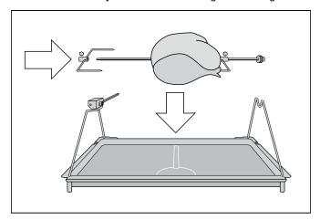
4. Plug the left retaining clip onto the rotisserie spit and screw it in firmly.
