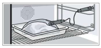
**Poultry:** Insert the core temperature probe as far as it will go into the thickest point in the breast. Depending on its structure, insert the core temperature probe into the poultry crossways or lengthways. With poultry, make sure that the tip of the core temperature probe does not protrude into the cavity in the middle of the bird.
